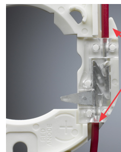
Molex solderless LED array holders utilize a dual wire trap to accommodate a poke-in-wire connection and allow LEDs to be daisy chained together
